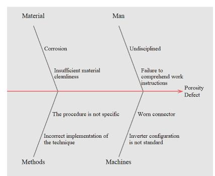
Figure 2. Fishbone Diagram for Porosity
