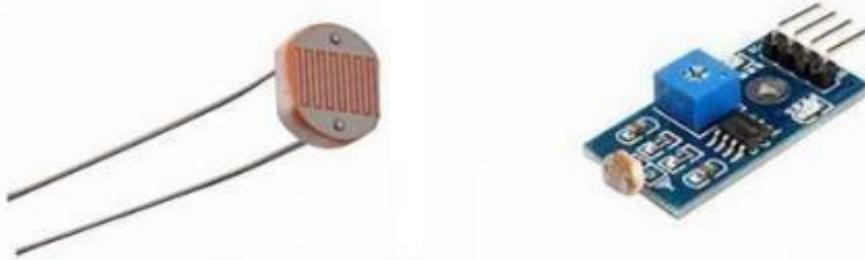
**Gambar 2.** Sensor Light Dependent Resistor
