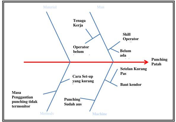
Gambar 5.3 Diagram Fish Bone Unplanned Down Time Punching Patah
