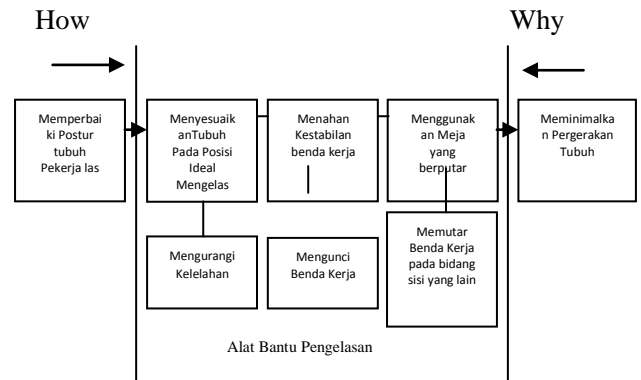
Gambar 2. Diagram FAST Alat Bantu Pengelasan
