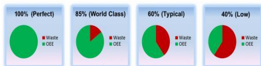
Gambar 2.7 Level Overall Equipment Effectiveness (Japan Institute of Plant Maintenance (JIPM))
