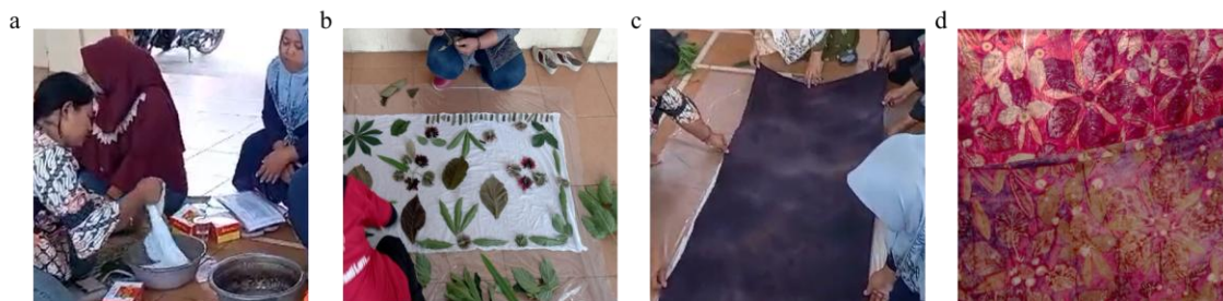
Figure 2: Ecoprint-making process during the training session. (a) Mordanting process (b) Arrangement of flowers and leaves (c) Cover fabric dipped in natural dye (d) Ecoprint results.
