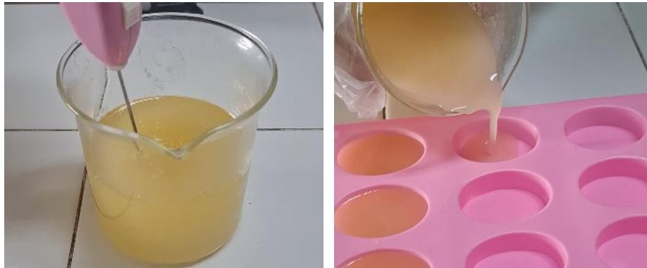
Figure 1. Mixing Process of Used Cooking Oil and Alkali Solution in Natural Soap Production
