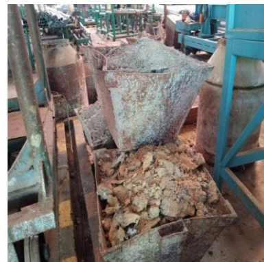
Gambar 8. Limbah zinc dross hasil zinc recovery
