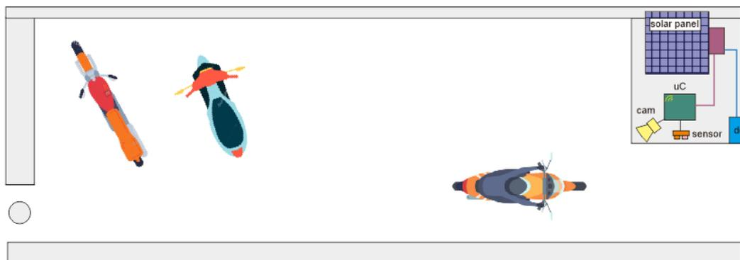
Figure 5. Monitoring System Set-up
