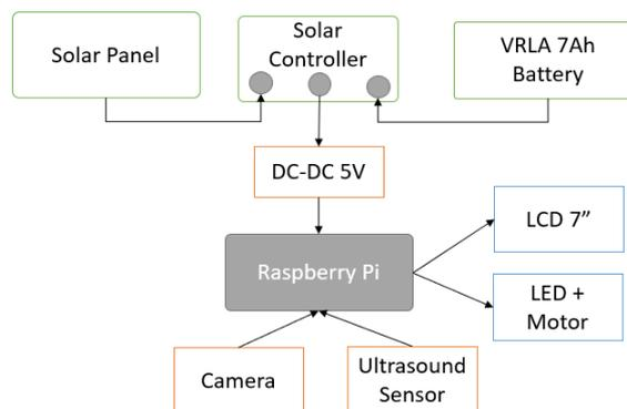
Figure 7. Hardware Connection of Monitoring System
