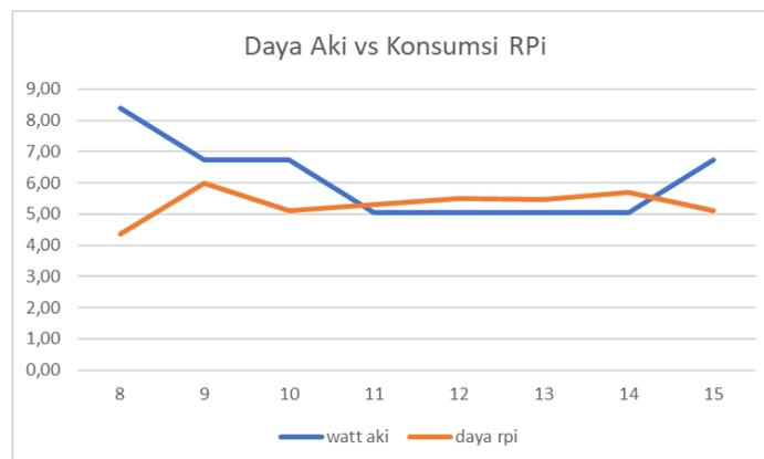
Figure 8. Comparison Chart of Battery Power with Raspberry Pi Power Consumption
