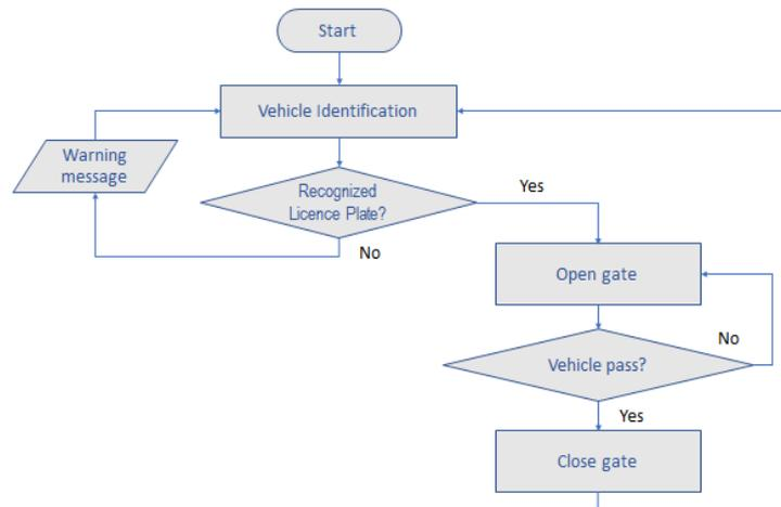
Figure 6. Working Diagram of Monitoring System
