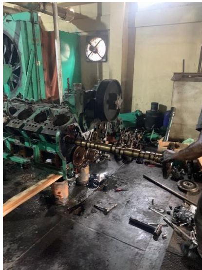
Gambar 7. Maintenance Camshaft mesin diesel Cummins KTA 38 G5
