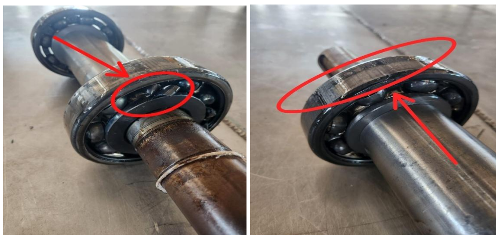
Gambar 8. Bearing Defect (Sumber, PT XYZ, 2025)
