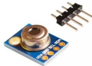
Gambar 1. Sensor Suhu Non Contact MLX90614 GY-906
