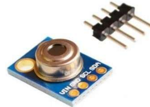
Gambar 1. Sensor Suhu Non Contact MLX90614 GY-906
