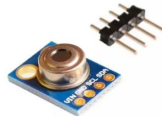
Gambar 1. Sensor Suhu Non Contact MLX90614 GY-906
