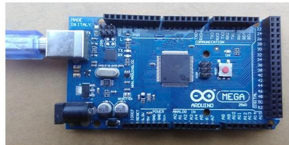
**Gambar 2.3** Arduino Mega 2560
