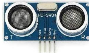
Gambar 4. Sensor Ultrasonik
