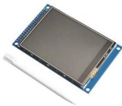
Gambar 6. LCD TFT
