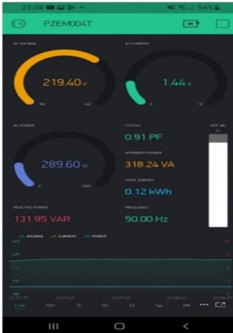
Gambar 5. Monitoring Tegangan
